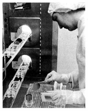
SILICON WAFERS containing 65 integrated circuit dies are loaded into quartz boats by Jean Green (2141) for high temperature processing. After processing, the dies are cut apart for assembly.
